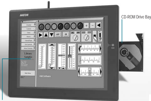
IP-65 certified front panel with touchscreen
