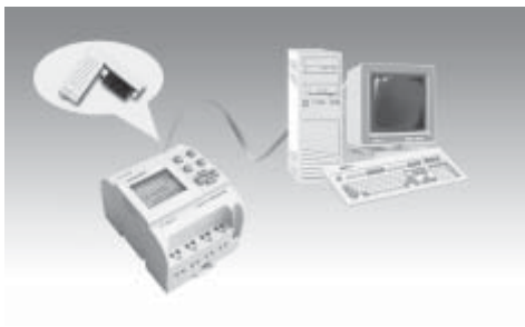
Fig. 4 . 24. FAB Communication Connection Frame
