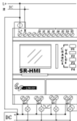
Fig. 2.12-2 The PNP Transistor Output
